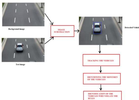
**Figure 2.** The block diagram of the proposed method
