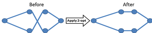
Fig. 7 Illustration of a 2-opt operation (reproduced from Karakaya 2015)
