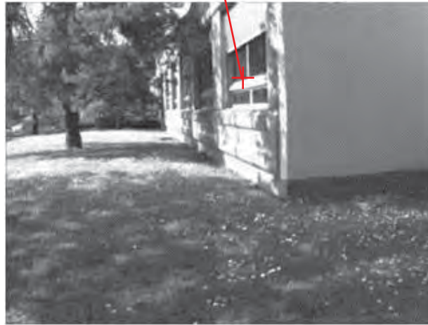
Figure 7. Another image is taken by the same mobile robot in another new position (x_r + \delta_x, y_r + \delta_y, \theta_r + \delta_\theta) in a moment (t + \delta t) ; the template matching is realized by searching the least local minimum which was detected in one point which is marked by a small red cross.
