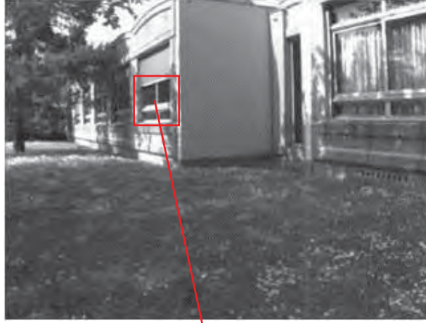
Figure 6. The first image is taken by mobile robot in the position (x_r, y_r, \theta_r) in a moment (t) , the template which is surrounded by red square, is selected as a part of the image that contains some important features
